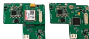
Radio LoRa and GPRS communication modules
