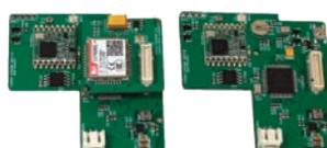
Radio LoRa and GPRS communication modules
